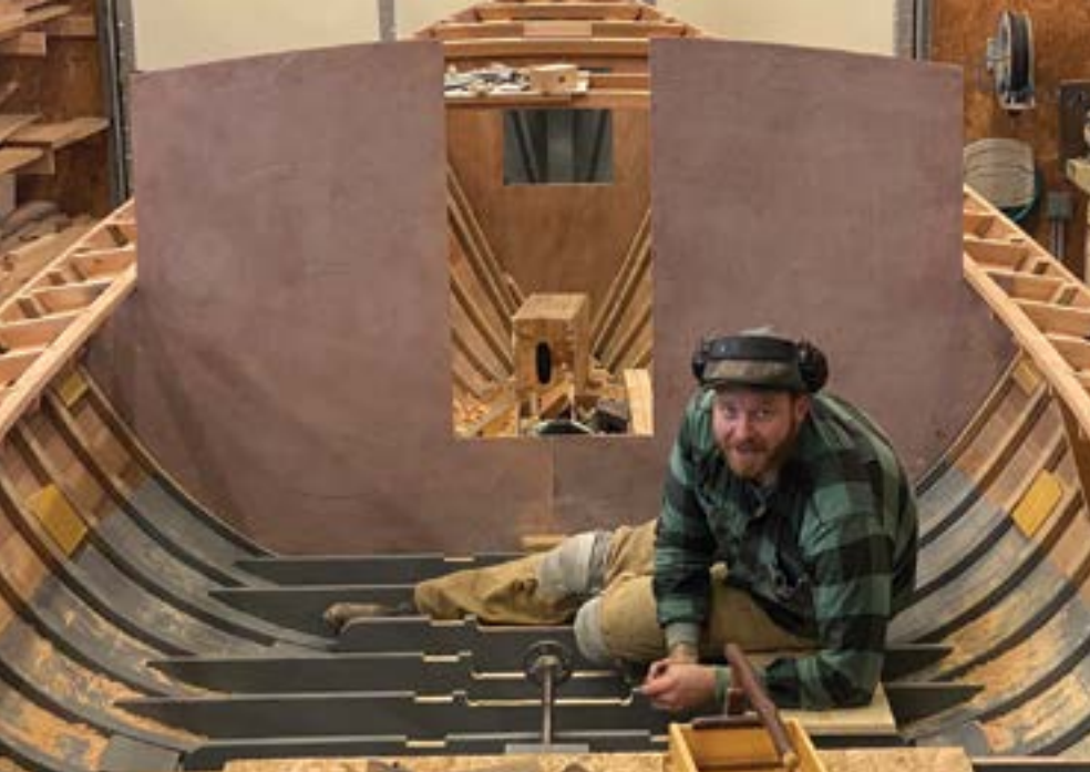
Boatbuilding student Jordan McIntosh fitting the engine beds for the lobster boat's 110hp Yanmar engine.
