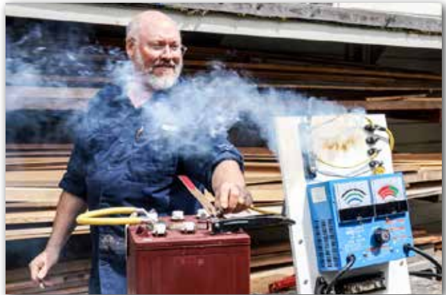
Instructor Kevin Ritz gives a demonstration on the importance of using the proper wire gauge.
