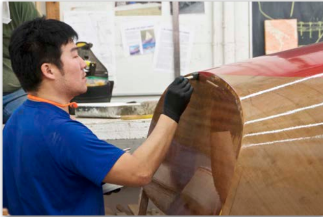
Student Seongho epoxies the transom of the cold-molded Kingston launch.
