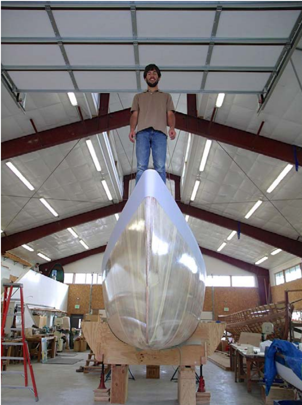
Standing on Sliver - a 62-foot sloop designed as a minimalist day sailor. Designed by the renowned designer Robert Perry for a client in the Pacific Northwest, it is a strip-planked, wood hulled, composite day sailor. This is the largest boat built at the school. It was constructed by Contemporary Wooden Boatbuilding students under the direction of Instructor Bruce Blatchley.
